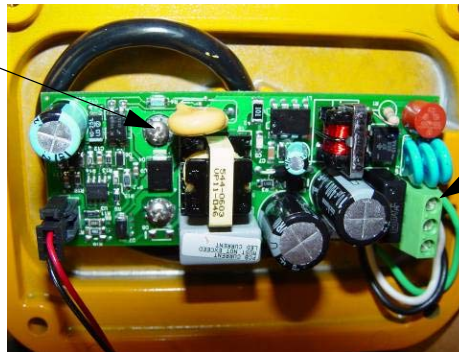
Figure 11: PCB Assembly Mounting Screws
