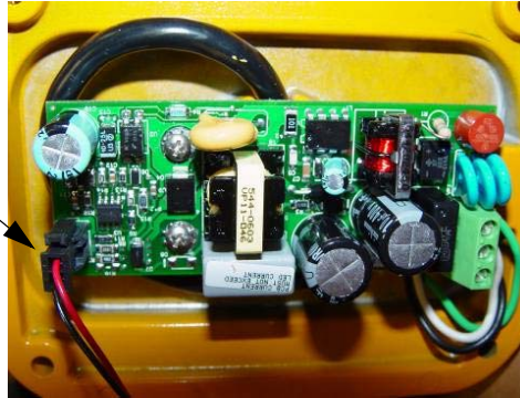
Figure 10: PCB LED Disconnect
